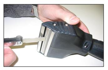
Figure 3-6. Clean the Solution Bar Jet
