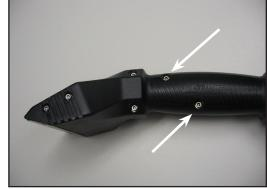
Figure 2-1. Remove Tool Screws
